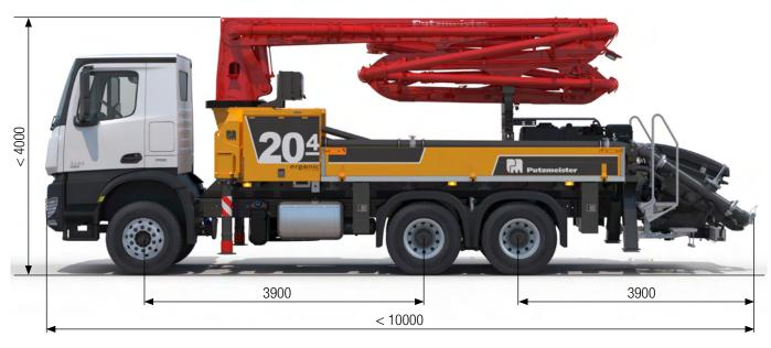
Note: Standard version. Dimensions and weights depend on truck, pump model and equipment. Dimensions in mm. Example based on Mercedes Benz Arocs 2636. For illustration only.
