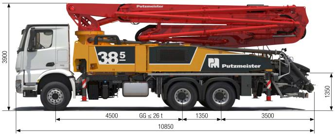
Note: Standard version. Dimensions and weights depend on truck, pump model and equipment. Dimensions in mm for MB 2640.
