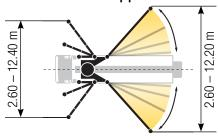
Dimensions can differ depending on configuration. Support width based on center of support leg. The specified values are reference forces.
