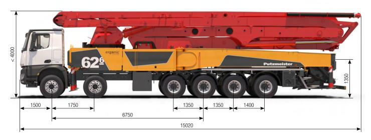
Note: Standard version. Dimensions and weights depend on truck, pump model and equipment. Dimensions in mm, MB-Arocs 6553 12x4 R6750 E6. For illustration only.
