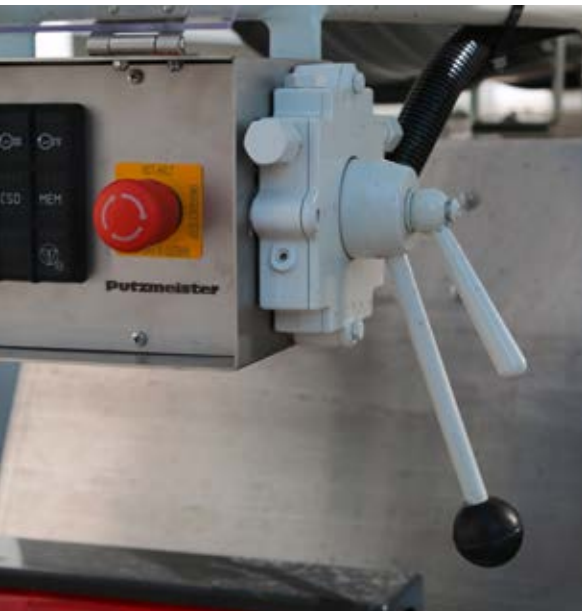
Operating lever for drum speed and rotational direction
